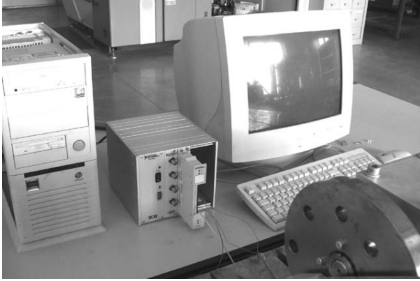
Figure 4: The acquisition system and the motor control system
