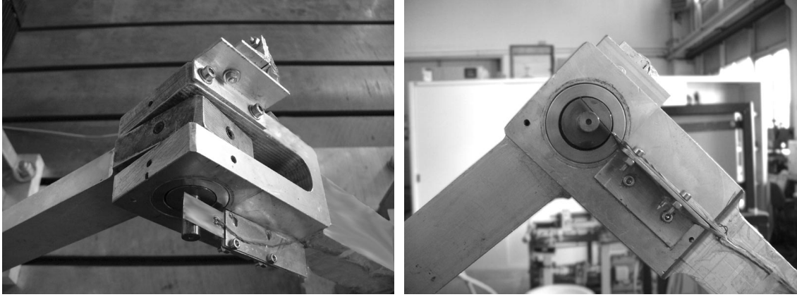
Figure 3: The measuring device, mounted on the revolute joint with clearance
